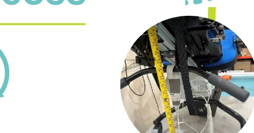
The load applied to each chair component is based on the specified load rating. The correct load is determined using pressure calculations, ensuring the pressure pad applies the appropriate load.
